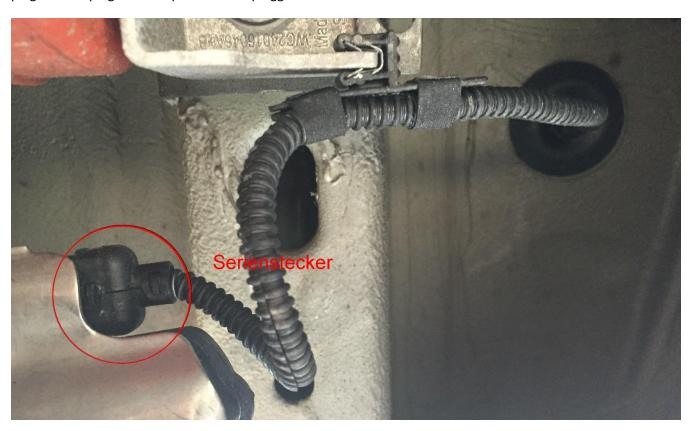
For cars with a servomotor left + right both Y-cables can each be mounted left or right, this has no influence the function of the controller.
