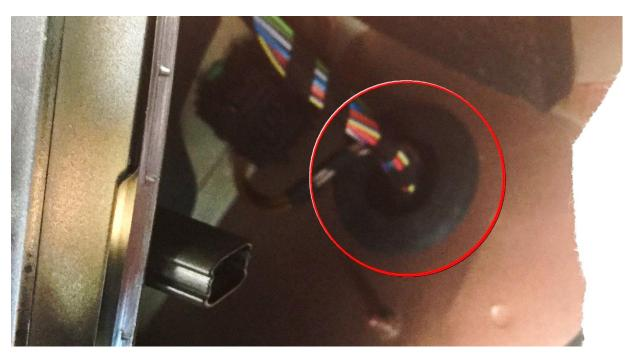
On the end the original connector has to be deducted from the servo motor, plugged into the appropriate mating plug and the plug of the flap control are plugged into the servomotor:
