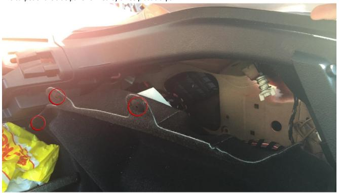
Behind the carpet, a controller maybe located. If so, he can be easily removed, he is only attached to one pin of the car body:
