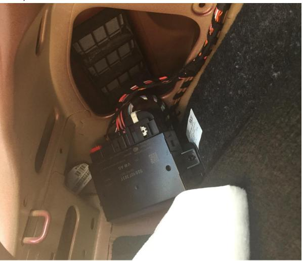
Now the rubber grommet is visible, the plug must be inserted through the rubber either or if this is not possible, be guided past the hole on the side:
