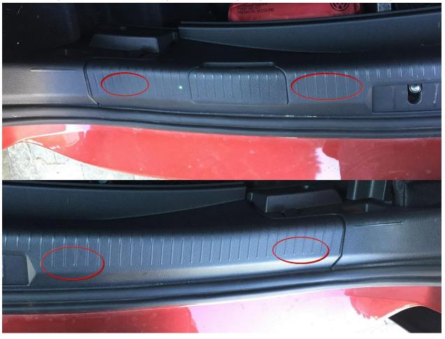
Unscrew the screws on the left and right for the side panel (Torx 25):
